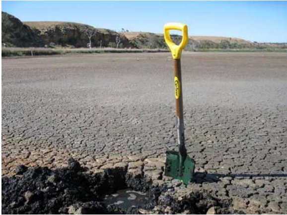
Figure 2. Monosulfidic material (or monosulfidic black ooze: MBO), in acid sulfate soil exposed in a shallow back swamp/wetland (Paiwalla wetland adjacent to the Murray River; Site E4 in Fig. 5; Fitzpatrick et al. 2008f). Monosulfidic material, if mobilized in water bodies, is able to rapidly remove dissolved oxygen from that water.
