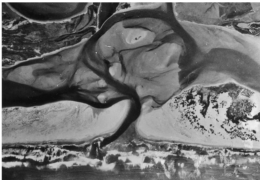
Fig. 11. Aerial photograph of the Murray Mouth showing flood tidal sedimentation in 1945, five years after barrage construction. Source: Mapland, South Australia.
